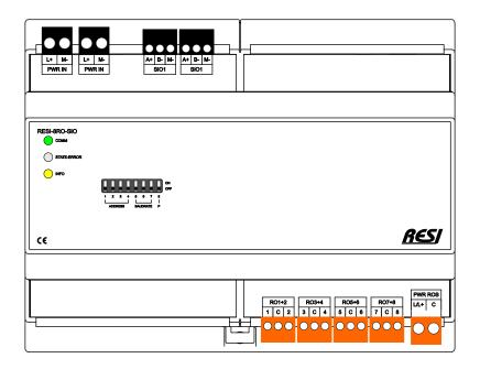
DIN EN 50022 Snap-on for DIN-Rail ON-WALL Mounting on-wall
